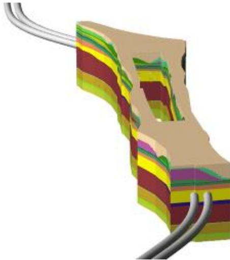
*Figure 3D geotechnical model*
