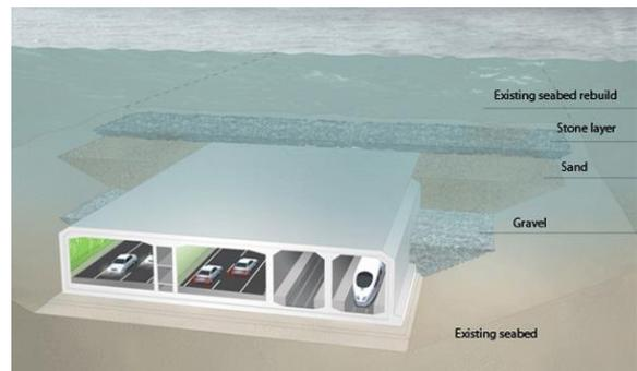
Figure: Tunnel location and typical cross-section
