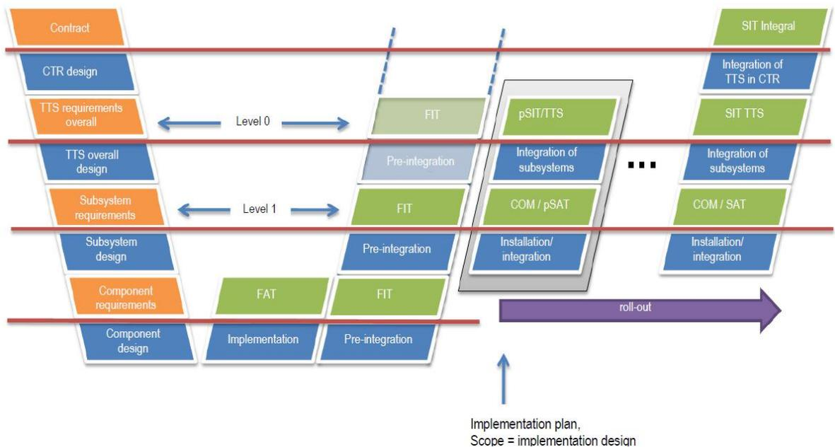
Figure V-model design traffic and tunnel systems 2nd Coentunnel.
