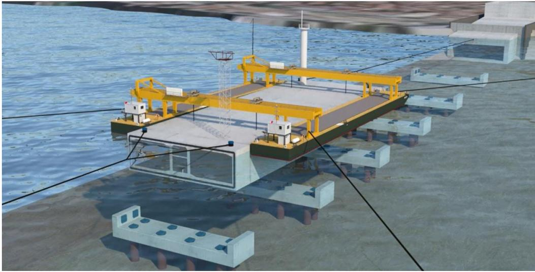
The geology in the Golden Horn is characterized by 30-40 m soft layers on top of weathered sandstone and siltstone. The riverbed is at 35 m below water level and considered deep. Due to the combination of steep slopes, dense population and the need to connect to the boulevards a tunnel below riverbed was not possible. A submerged tube bridge was therefore the most suitable option. For local shipping a navigation channel of 8.5 m deep and 300 m wide had to be accommodated.
