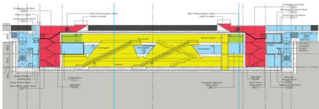
For reasons of controlling the climate and passenger safety the Client required to design for Platform Edge Screens. In this way the trainway is physically separated from the platform thus creating a comfortable climate on the platform.
