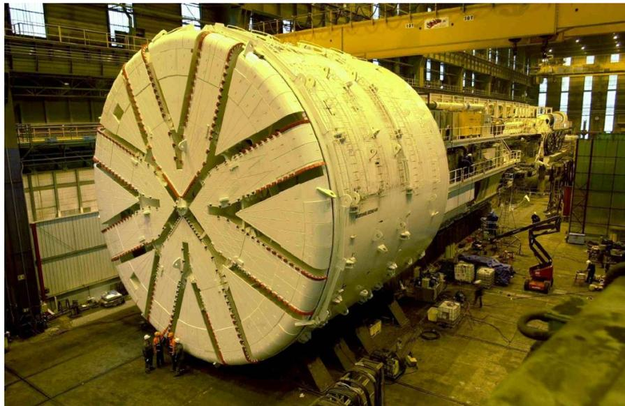
*Figure: The 14.5m diameter TBM for the Groene Hart tunnel*
